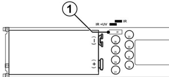
Fig. 7-2 1. (1) Positions of the internal jumper IR + UV
