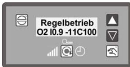
Fig. 7-2 CO control display
