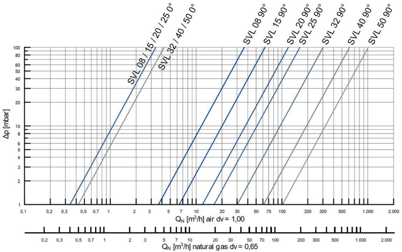
Fig. 5 Flow curve gas control valve 668M2400
