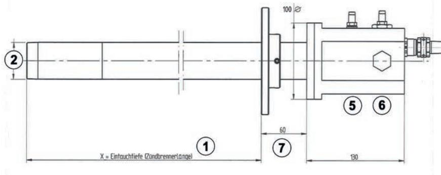
Dimensions of GFI48 pilot burner design C Safe Area
