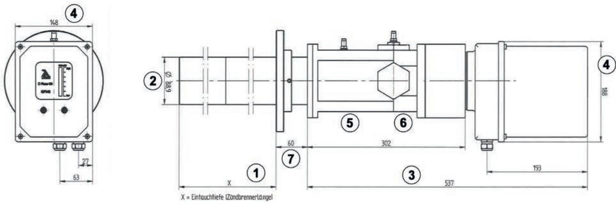
Dimensions of GF170 pilot burner design A/B
