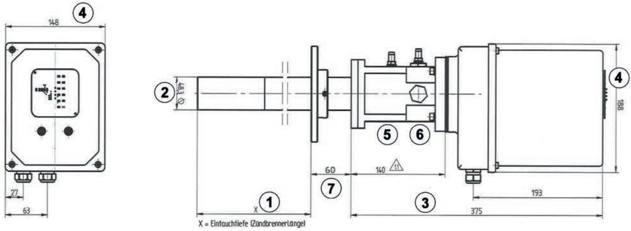
Dimensions of GFI48 pilot burner design A/B
