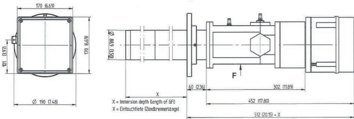
Dimensions of GF170 pilot burner Ex-Zone 2
