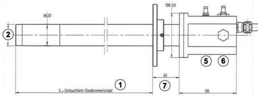
Dimensions of GF135 pilot burner design Safe Area
