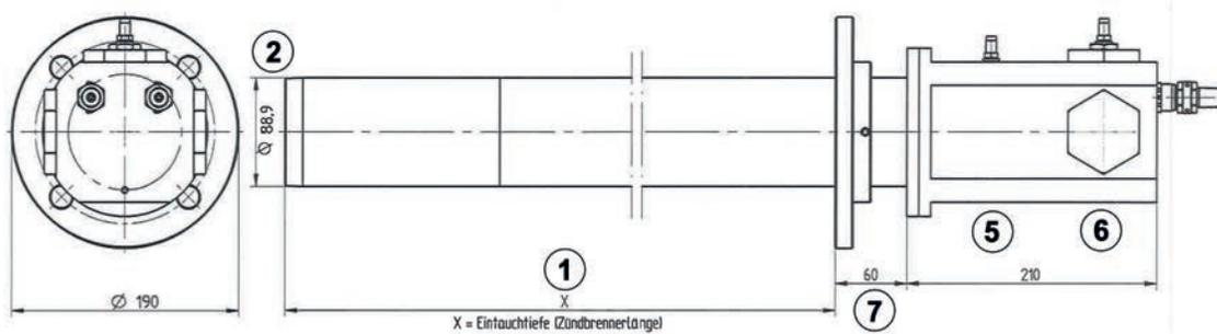
Dimensions of GF189 pilot burner design C Safe Area
