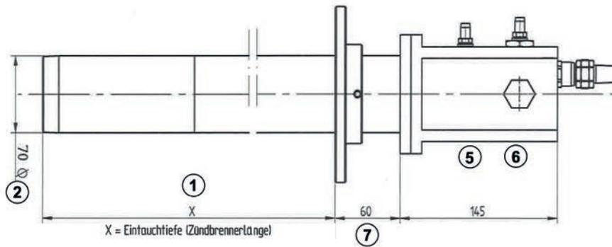
Dimensions of GFI70 pilot burner design C Safe Area
