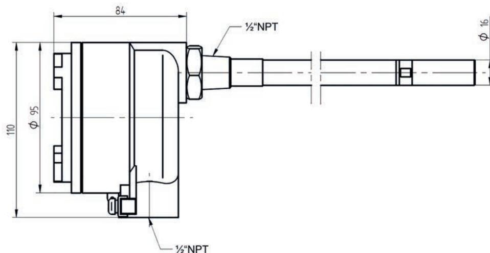
Dimensions of the ignition lance with aluminium connection box
