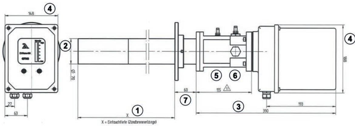
Dimensions of GFI70 pilot burner design A/B
