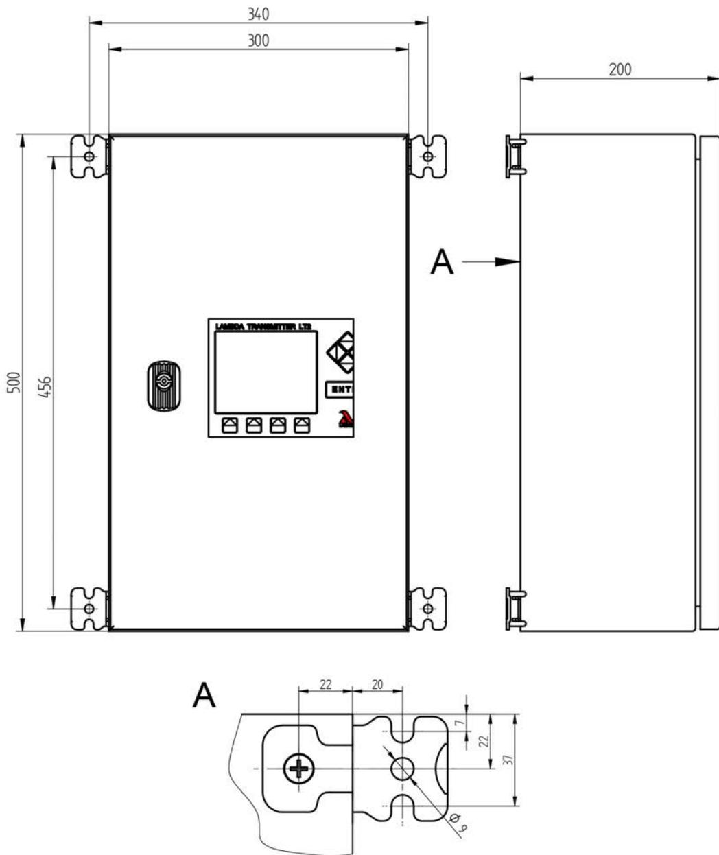
Fig. 4 Dimensional drawing LT2 in wall mounting housing with reference air pump
