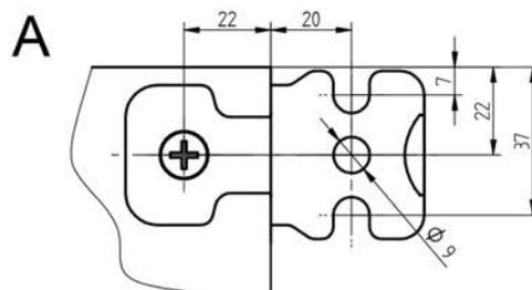
Fig. 3 Dimensional drawing LT2 in wall mounting housing
