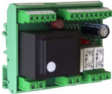
Fig. 10-3 FN20 Top hat rail mounting
